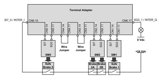
Both [SQ3 function assignment] 5 [ 12 and [SI7 function assignment] 5 [ 13 of each chained safety module are set to SBC Feedback.
