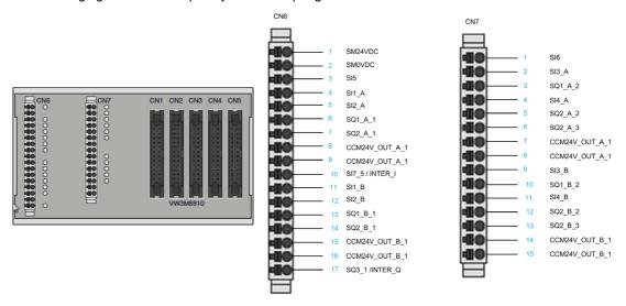
NOTE: A sticker is provided with the Terminal Adapter for CN6-CN7 pin arrangement.
