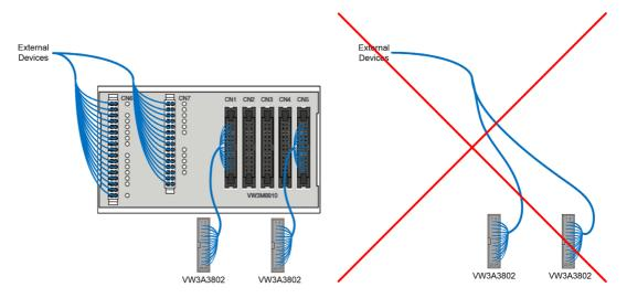
Use of several safety modules with a terminal adapter implies to have a consistent configuration between the connected safety modules. For example, but not limited to, a consistency between the configuration of the inputs and outputs of each safety module.
