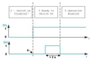
SIx Inputs assigned to the safety function SS1
