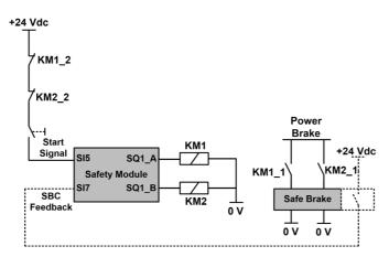
SBC feedback signal (dotted line) is an optional signal.
