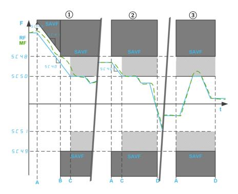
F: Frequency / RF: Reference Frequency / MF: Motor Frequency
