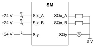
Slx\_A and Slx\_B: Safety Input x (Channel A and B)
