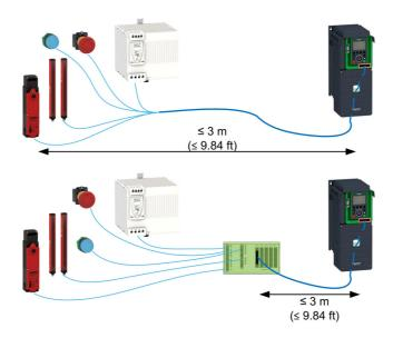
Verify that the wiring, cables, and connected interface meet the PELV (Protective Extra Low Voltage) requirements.
