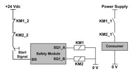
The wiring of KM1\_2 and KM2\_2 contacts on the start signal helps to prevent the start of the safety module in case of welding contacts on the power contactors KM1 and KM2 if KM1\_2 and KM1\_1 are mechanically linked but also KM2\_2 and KM2\_1.
