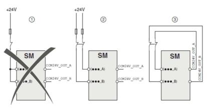
There are three ways of connecting the signals to the safety module
