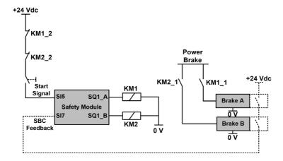
SBC feedback signal (dotted line) is an optional signal. The wiring of KM1\_2 (or KM2\_2) contact on the start signal helps to prevent the start of the safety module in case of welding contacts on the relay KM1 (or KM2) if KM1\_2 and KM1\_1 (or KM2\_2 and KM2\_1) are mechanically linked.
