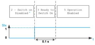
SIX Inputs assigned to the safety function SS1
