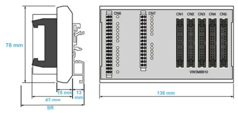
SR Space requirement (with cables connected to CN1...CN5): cable + 42 mm + 13 mm ≥ 100 mm.
